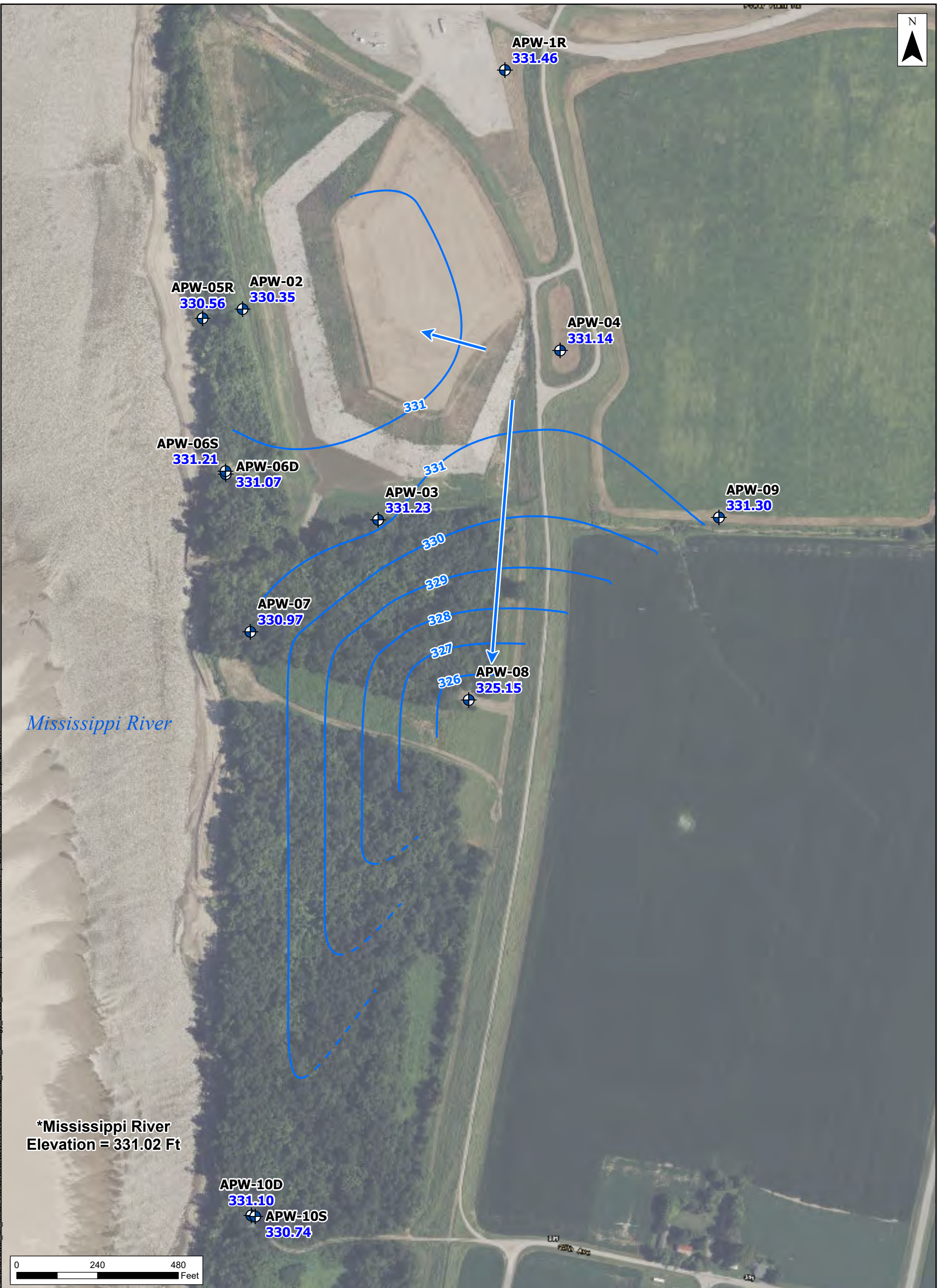
Figure 2: First Quarter 2024 Groundwater Contour Map Grand Tower Energy Center, LLC Grand Tower, Illinois Jackson County
