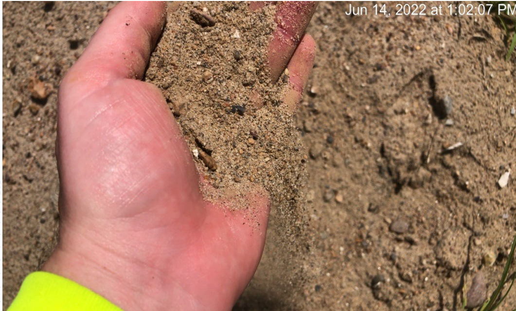
Close-up of exposed GTEC levee material.
