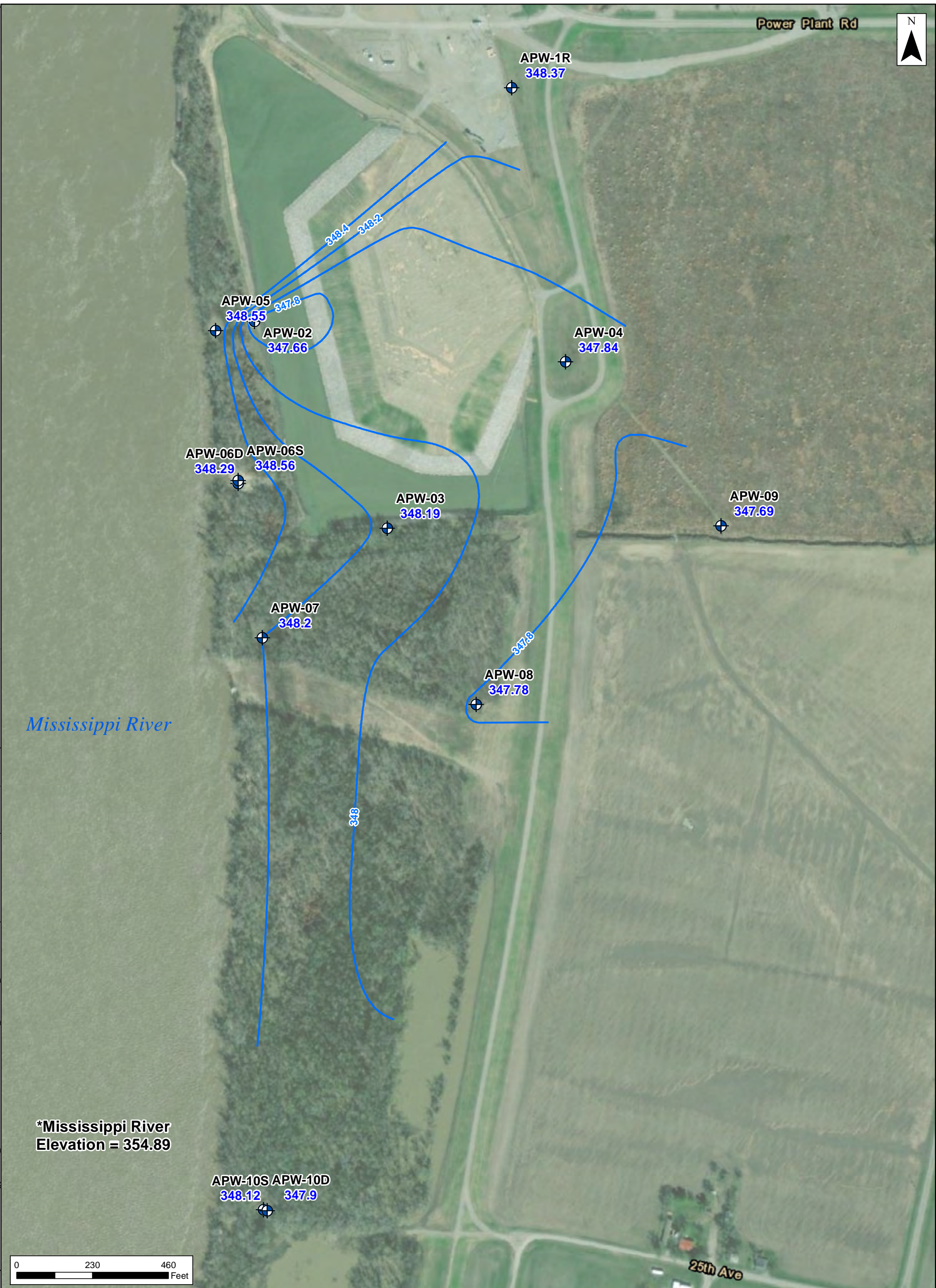
Figure 6 Monitoring Well Locations and Groundwater Contour Map June 2022 Grand Tower Energy Center, LLC Grand Tower, Illinois Jackson County
