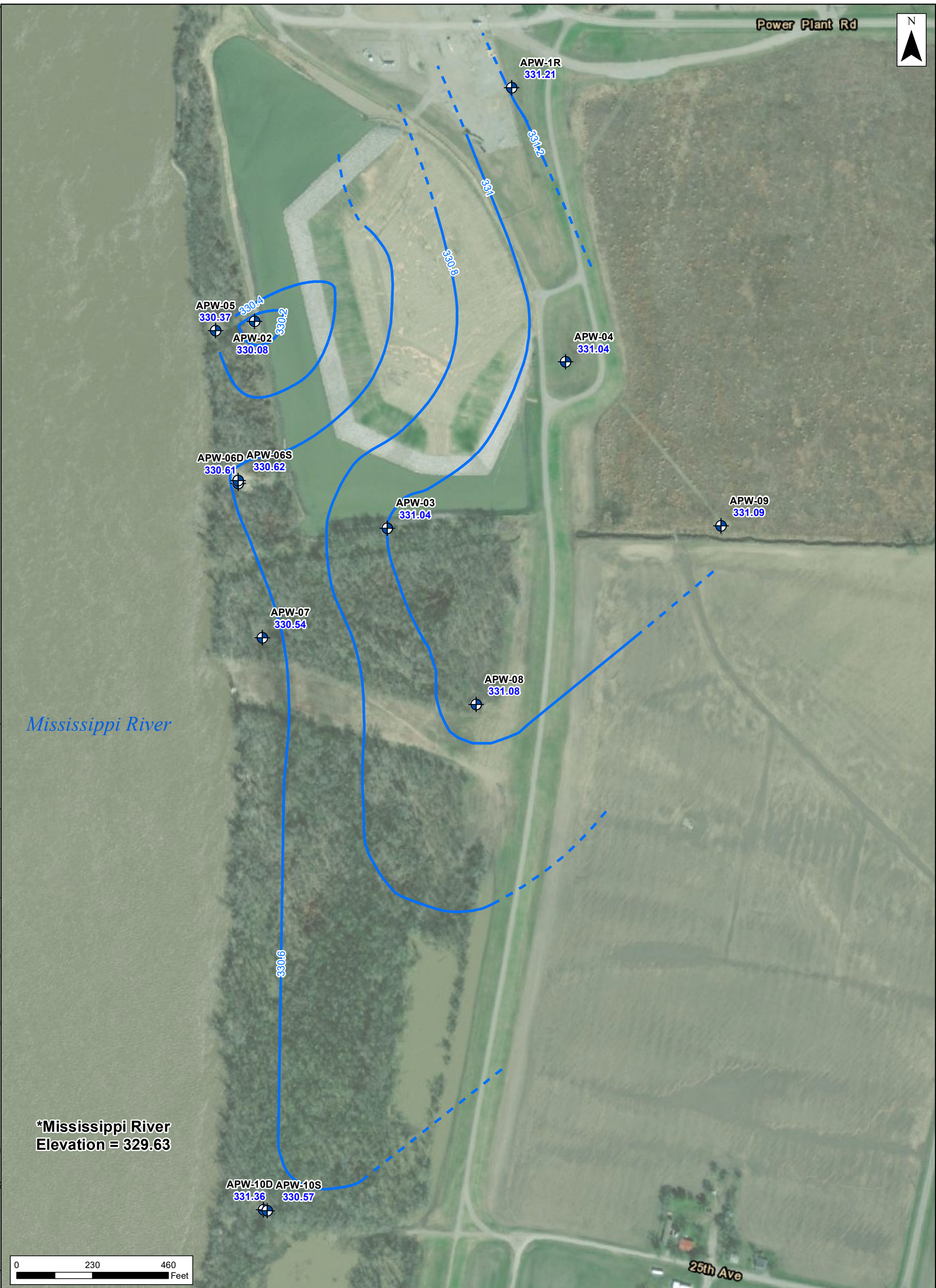
Figure 8 Monitoring Well Locations and Groundwater Contour Map November 2022 Grand Tower Energy Center, LLC Grand Tower, Illinois Jackson County
